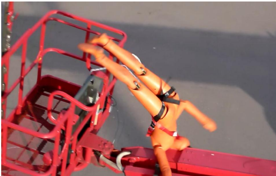
Figure 2: Fall sequence from telescopic work platform due to catapult effect (whiplash effect) and use of a lanyard which is too long → Videos under www.bauforumplus.eu/absturz
