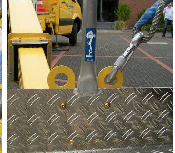
Figure 4: Always use the anchor points as specified by the manufacturer of the work platform (> 3kN). Position anchor point: Near to ground, maximum height medium rail. Never secure to the railing!
