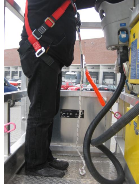
Figure 3: Securing means as short as possible when moving the work cage → adapt rope adjuster!
